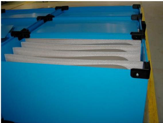
These returnable totes were designed to protect sensitive cosmetic or “class A” surfaces on vinyl automotive interior parts. In the previous expendable packaging, the parts had to be individually poly bagged to protect class surfaces from the abrasive corrugated packaging. While Milform’s® corrugated plastic is non-abrasive to cosmetic surfaces, foam can still be added to the dunnage to act as a buffer to the part surfaces.
