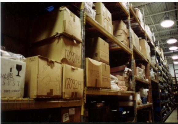
Before implementation of Milform® bins, parts were stored in a mixture of corrugated containers and molded plastic bins of many sizes.
