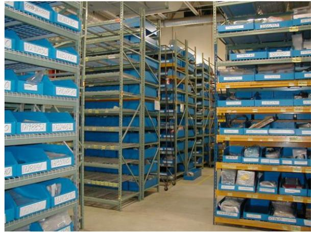
The results were total warehouse space savings of 40% by replacing the existing standard molded bins with custom Milform® bins. Custom Milform® bins added extra 5 shelves per rack. This addition to vertical storage consolidated warehouse space while increasing pick locations by 1,250 (see picture below).
